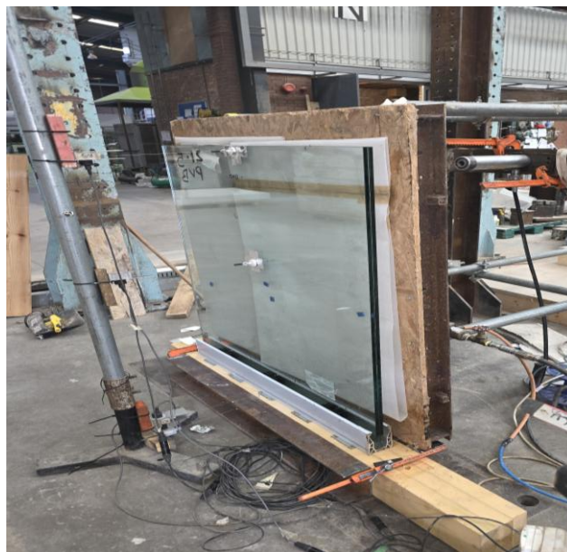
Plate 2 – Generic Test Configuration Uniformly Distributed Load
