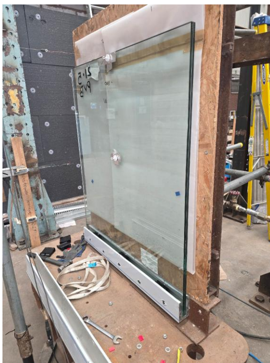
Plate 2 – Generic Test Configuration Uniformly Distributed Load
