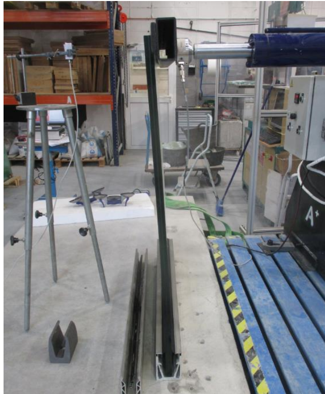
Horizontal static test, outwards ( 3,0 kN/m )
